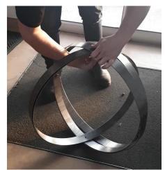
Spread the 3 rings around so that they are evenly spaced top and bottom with 60 degrees between each ring.
